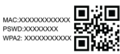
**Your SSID** (The network name you should connect to) will be **“AirCube-XXX”** where **“XXX”** **represents the last 3 alpha-numeric (Letters and Numbers) of the MAC portion of this label.** The Wireless Password that should be used to connect your laptops and phones will be the letters and numbers to the **right** of the **“WPA2”** label. Note that the password is **CASE SENSITIVE**. This means that upper-case and lower-case matter!
